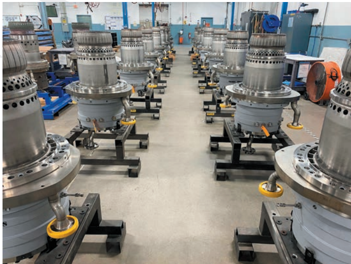
501F FlameSheet™ ready to be sent to site for 2020 installation along with PSM's 501F GTOP7
